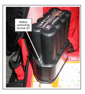
5. After arriving at your destination, re-attach the battery and turn the system on briefly to check the battery status and perform a self-diagnosis according to the JetForce Backpack Instructions For Use.
